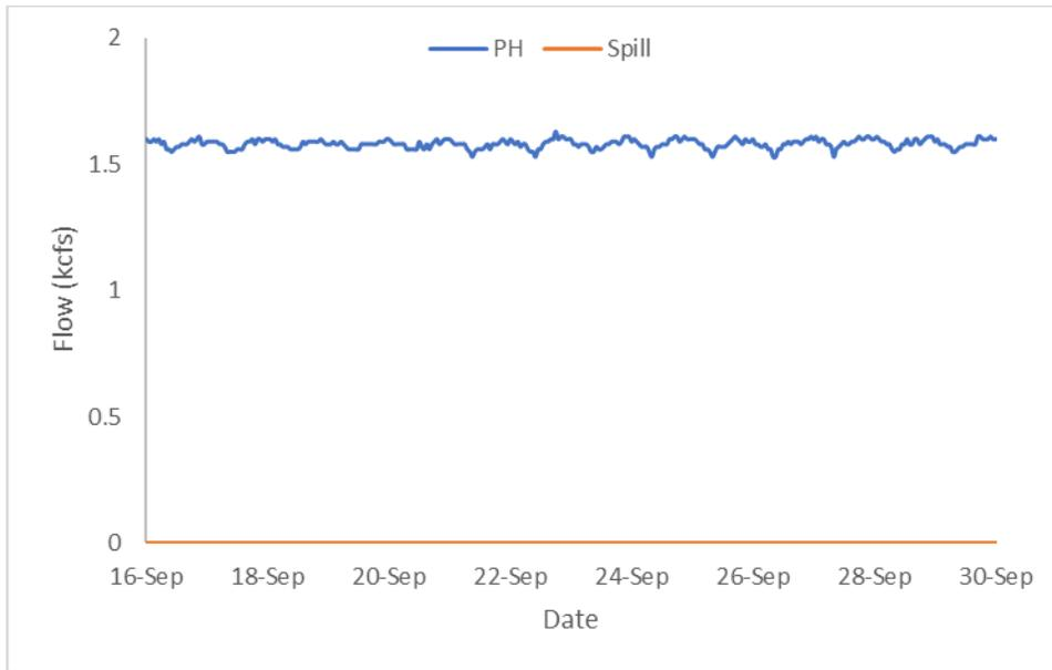
**Figure 15. Hourly Flows PWR vs. Spill (Big Cliff Dam)**
